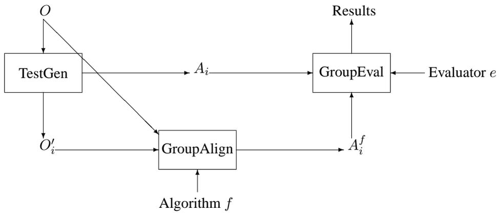
Figure 4.2: Process flow provided by the tool suite.
